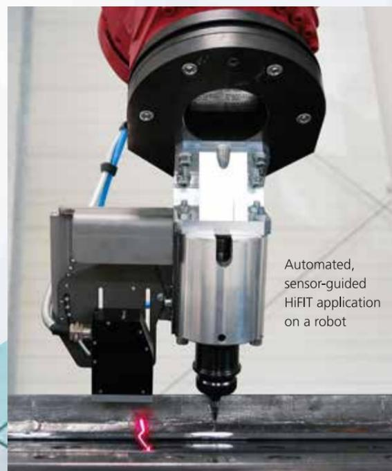
Automated, sensor-guided HiFIT application on a robot
