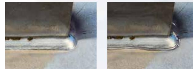
Before / after: Thanks to the HiFIT method, the weld fatigue limit is improved by 80% to 100%!
